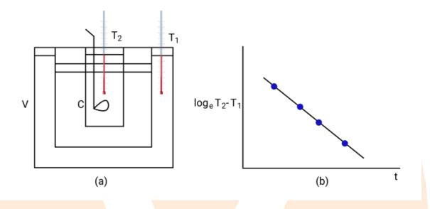
**Configuration:** A double-walled vessel (v) with water contained between two walls.
