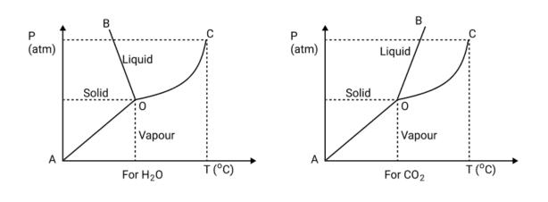
Line AO is the sublimation curve, line OB is the fusion curve, line OC is the vapourisation curve, point O is triple point, point C is critical temperature
