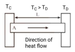
The rate of heat energy flowing through the rod becomes constant at steady state. It is given by,
