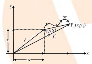
Now, if the particle moves along the path as shown to a new position  $P_1$  with the position vector  $\vec{r}_1$ ;
