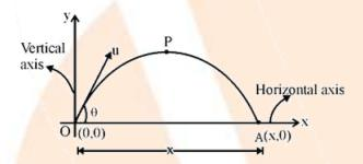
Here, a particle is projected at an angle with an initial velocity 'u'.
