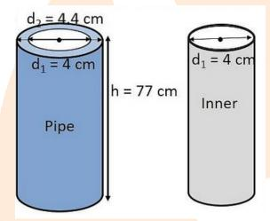
Inner diameter of cross-section = 4cm
